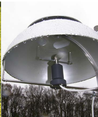
Fig 1.3 Rotating-arm sampler with detachable arms operating in wet conditions in 2012
