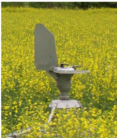
Fig 1.2 Burkard seven day spore trap operating in an oilseed rape field at Rothamsted
